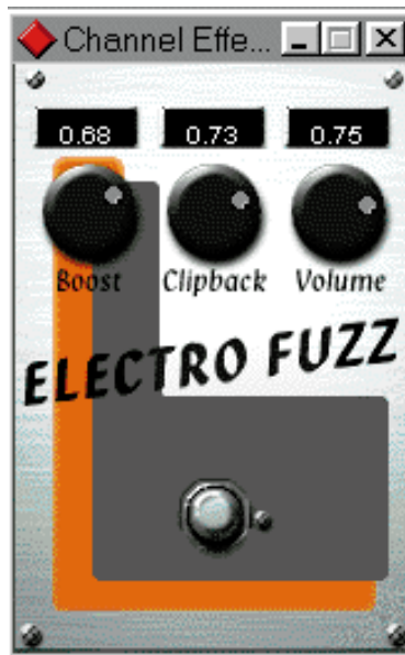
Fig 2 (right) Electro Fuzz takes mono input from a mixer effect and distorts it
